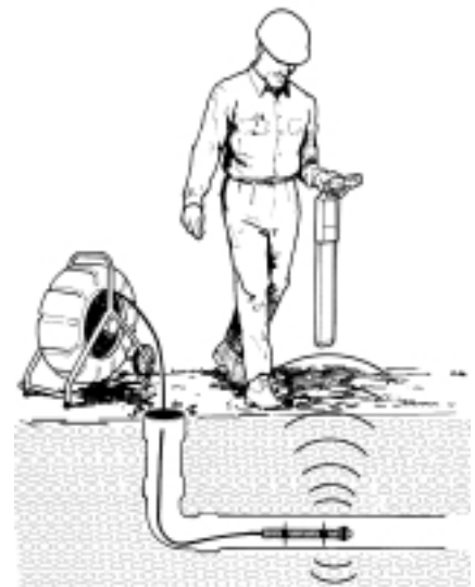
The Pointer™ XL and SeeSnake™ with In-Line Transmitter identify and accurately locate problems in the line.
